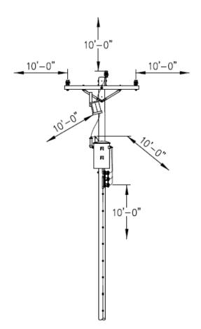
Keep a 10-foot clearance from any energized electric part for voltage less than 50 kilovolts.
